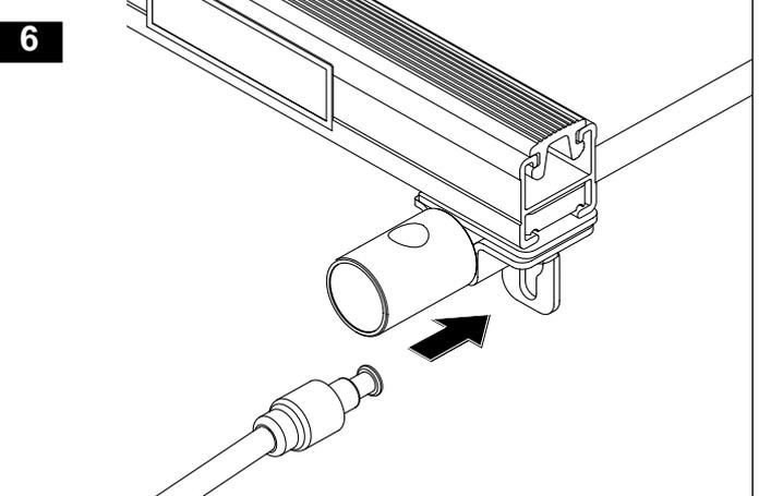
To lock cable lock, key must be in lock. Then insert locking pin and remove key. To unlock insert key, turn and remove locking pin.
