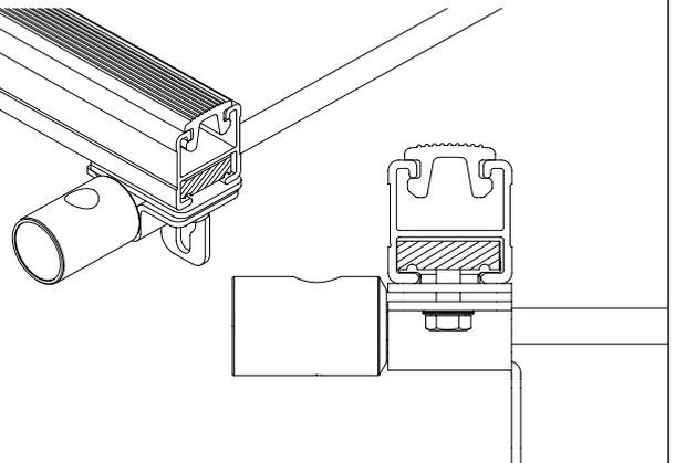
Position the cable lock and bracket assembly, tighten the screw to 5-6Nm to secure the bracket. Peel and stick the yellow warning labels onto the crossbar adjacent to the cable lock.
