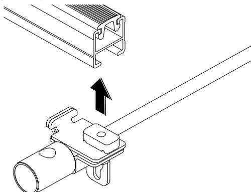
Check that the lock housing is facing the rear of the vehicle, turn the channel nut so that the channel nut is fully located across the crossbar.
