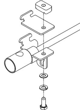
Insert the T-shaped lugs on the brackets into the underside of the crossbar. Turn the cable lock and bracket assembly so that the lugs engage the crossbar and the channel nut goes up into the crossbar recess.
